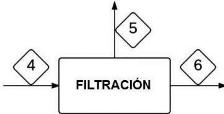
$$\begin{aligned} \text{Corriente 4} &= \text{Corriente 5} + \text{Corriente 6} \\ \text{Corriente 4} &= \text{LicorMadre (sulfatodeamoniosobresaturado)} \\ \text{Corriente 5} &= \text{LicorMadre} \\ \text{Corriente 6} &= \text{SulfatodeAmonioHúmedo (cristal)} \end{aligned}$$
