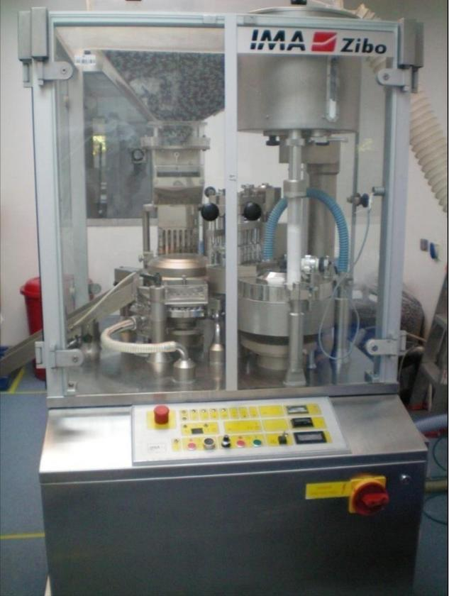
A photograph of an IMA Zibo Zanasi 40 F automatic capsule filling machine. The machine is a large, industrial-grade piece of equipment with a stainless steel body and a control panel on the front. The control panel features a red emergency stop button, several indicator lights, and a digital display. The machine is enclosed in a protective metal frame with a glass viewing window. The IMA Zibo logo is visible on the top right of the machine's frame. |
