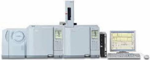
A laboratory chromatograph system consisting of a main unit with various gauges and a computer monitor displaying data. |
