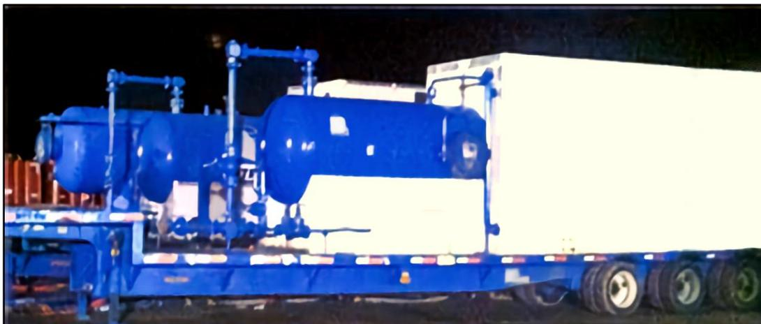
**Nota.** Tres separadores trifásicos en paralelo. Operaciones de *well testing* Tomado de *Hydraulic Fracturing in Unconventional Reservoirs*. <https://www.sciencedirect.com/book/9780128498712/hydraulic-fracturing-in-unconventional-reservoirs>
