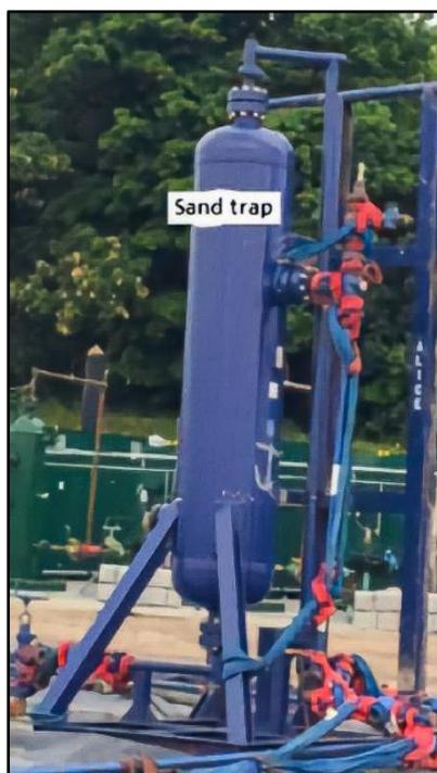
**Nota.** Líneas de superficie conectadas a trampa de arena. Tomado de Hydraulic Fracturing in Unconventional Reservoirs. <https://www.sciencedirect.com/book/9780128498712/hydraulic-fracturing-in-unconventional-reservoirs>
