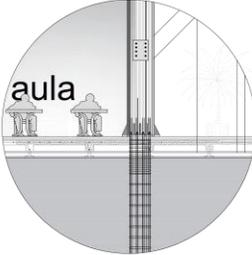
**UNION DE COLUMNA EN CONCRETO CON ESTRUCTURA METALICA**
