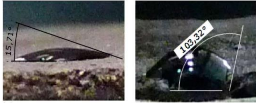
Figura 27 Contact angle change through treatment with 100ppm of aluminum oxide nanoparticles solved into SDS surfactant aqueous solution from J. Giraldo, P. Benjumea, S. Lopera, F. B. Cortés, and M. A. Ruiz, Wettability alteration of sandstone cores by alumina-based nanofluids, doi: 10.1021/ef4002956
