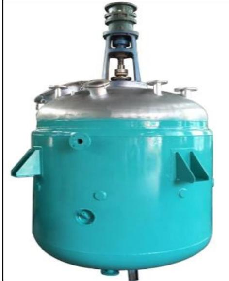
*Nota.* Se usa en el proceso de hidrólisis ácida y en el proceso de precipitación de la pectina. Tomado de: [https://spanish.alibaba.com/product-detail/china-batch-reactor-price-agitated-tank-reactor-fixed-bed-reactor-with-ce-62245689878.html?spm=a2700.md\\_es\\_ES.maylikeexp.1.3ea87f3bHW45Ar](https://spanish.alibaba.com/product-detail/china-batch-reactor-price-agitated-tank-reactor-fixed-bed-reactor-with-ce-62245689878.html?spm=a2700.md_es_ES.maylikeexp.1.3ea87f3bHW45Ar)
