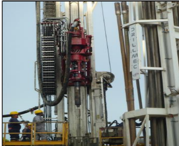
Figura 6. Hydraulic TDS, DRILLMEC (26035ft-lbs)
